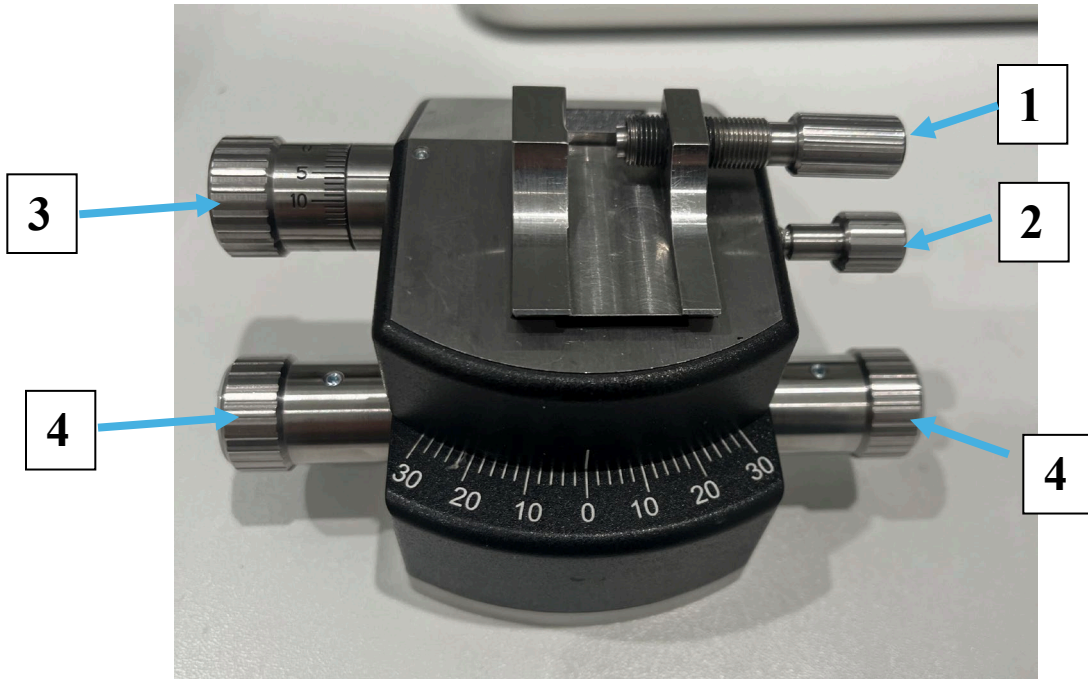
Figure 6. Labeled parts of the knife holder.
