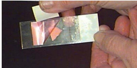
*Figure 20. Technique for removing Tape from Slide.*
