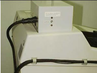
**13 Mech/Flash Unit Cable connected to ECU**
