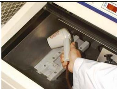
**04 Heat left wall for Mech/Flash Unit & Oil Bath placement Also heat the exposed adhesive on the mounting plate and oil bath**
