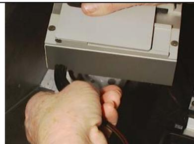
**06 Route Oil Bath & Mech/Flash Unit Cables underneath Mech**
