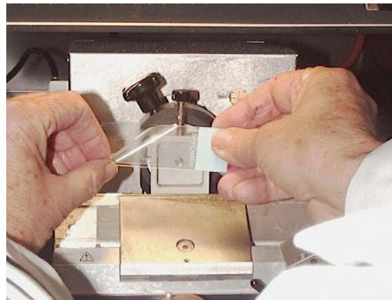
*Figure 7. Peeling mylar from adhesive coated slide.*
