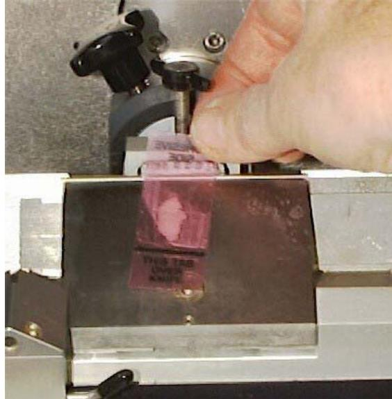
*Figure 13. Handling the cut section.*
