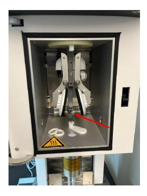
Before powering up the Vitrobot, check to make sure no forceps were left inside the machine!
