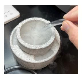
When you dispense the ethane, the gas can make it hard to see. Make sure your fingers are a safe distance away from the ethane as liquid ethane can cause severe burns!
