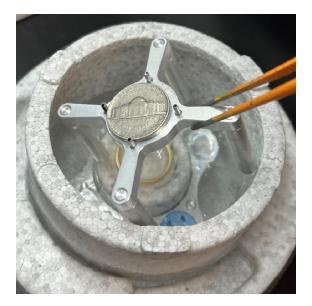
Remove the spider device with forceps. Caution! The metal spider device will be very cold and can cause severe burns if it contacts your skin.
