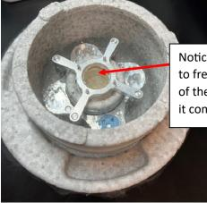
Notice the ethane starting to freeze around the edges of the brass cup. Don't let it completely solidify!
