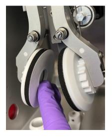
Clamp the filter paper against the blotting pad using the white plastic rings.
