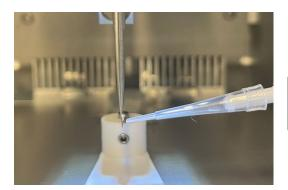
Pipette 3.5 μl onto the carbon-side of the grid.
