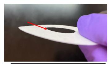
The backside of the filter paper has its edges frayed upward. This side goes against the blotting pad.
