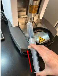
Connect the syringe to the tubing and inject the water into the humidifier reservoir.
