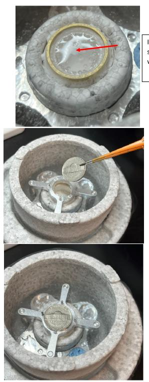
If there is a film floating on the surface of the ethane, blot it away with filter paper.
