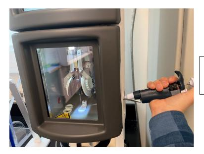
Apply sample through one of the side ports of the temp/humidity chamber.
