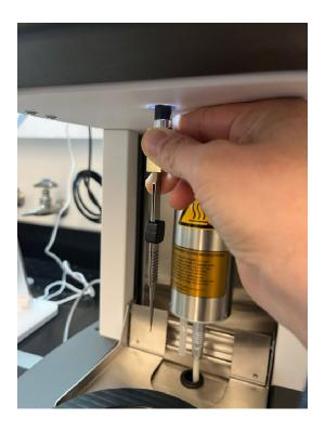
Ensure the Vitrobot forceps are properly engage with the arm to avoid a jam.
