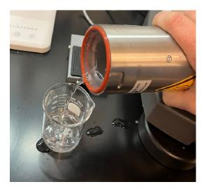
Remove water from the humidifier and leave the empty humidifier beside the Vitrobot to air dry.
