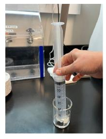
Fill the syringe to 60ml with **distilled water**.
