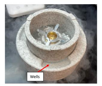
Start cooling the assembly by first pouring  $LN_2$  directly into the brass cup. As you pour the liquid nitrogen, the Styrofoam ring will rise. Once the violent bubbling has subsided it has reached  $LN_2$  temperature. Maintain the  $LN_2$  level so that the  $LN_2$  fills the wells of the Styrofoam cup by pouring  $LN_2$  into the wells of the Styrofoam cup (not into the brass cup).
