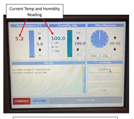
Wait for the temperature and humidity to reach the desired set points. It can take 20-30 min.
