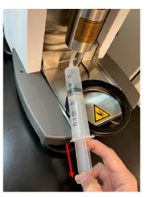
Once all the water has been injected, pull back on the empty syringe to create a vacuum.
