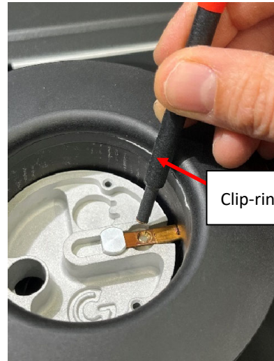
Remove clip-ring and any grid that may be in the holder.
