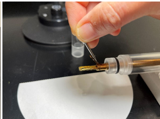
Use the pin to lift the grid clamp
