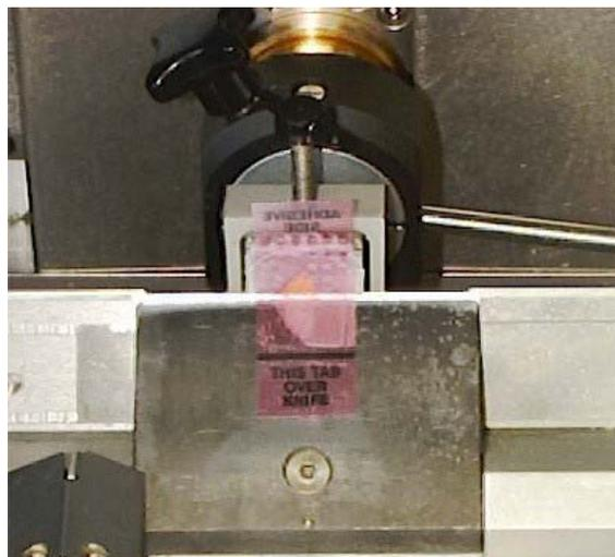
*Figure 12. Cutting the section.*
