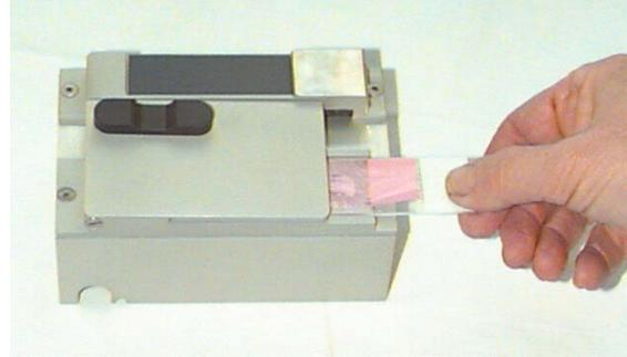
*Figure 16. Placing the slide into the Flash Tray.*
