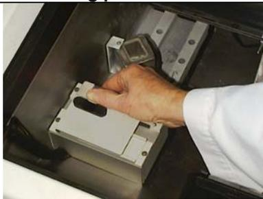
**\*07 Place Mech/Flash Unit in Chamber. Place Mech/Flash Unit low in chamber near the front wall. (Placement near the freeze bar is ideal in most cryostats)**
