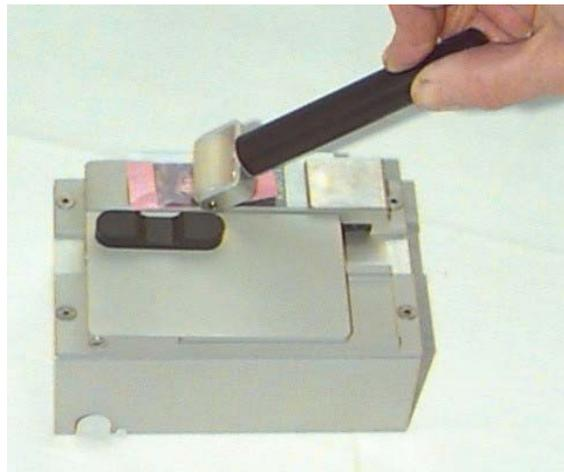
*Figure 15. Laminating the section to the Slide.*
