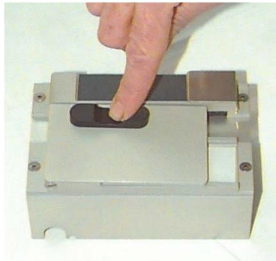
*Figure 17. Curing the adhesive on the Slide.*
