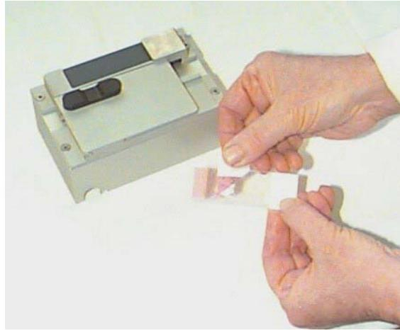
**Figure 19.** Removing Tape from cured Slide.
