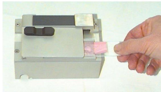
*Figure 18. Removing the cured Slide.*
