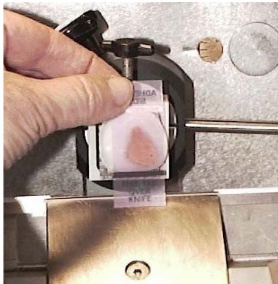
*Figure 10. Placing Tape on block face.*
