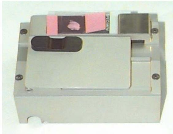
*Figure 14. Positioning the Tape on the Slide.*
