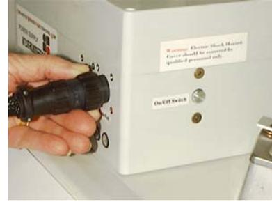
**12 Connect Mech/Flash Unit, Oil Bath Cables to ECU & Power cord to the ECU and wall outlet Turn the ECU on**
